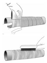
Apply compression film in the same direction as the 2 previous layers, starting beyond the outer edge of the *POLYGUARD IRO*, pulling firmly during application. Apply 2 layers of compression film over the entire composite area.
