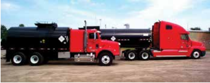
▲ Fill-Coat® #1 hot-installed casing filler is transported and heated in large tankers.
