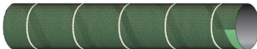
1. Start wrapping the pipe moving along the length of the pipe, so that the RockGuard overlaps slightly.
