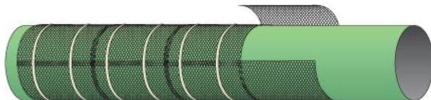
1. Cut the RockGuard into pieces of more than 6" extra than the circumference of the pipe.
