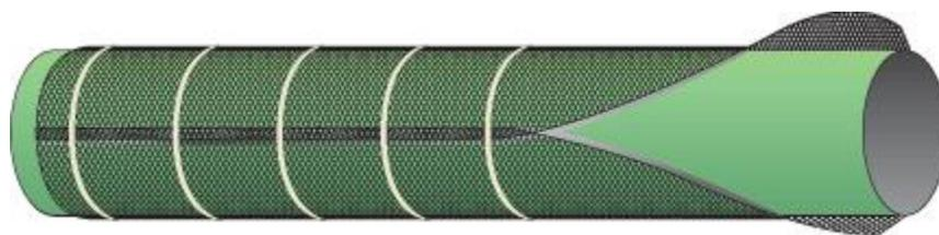
1. Unroll the mesh parallel to the pipe which is to be protected.
